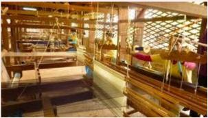
The final step is weaving. Silk weaving creates a fabric by interlacing the yarns. Weaving can be carried out on either a hand or power loom. Both hand and power looms are used in India today.
